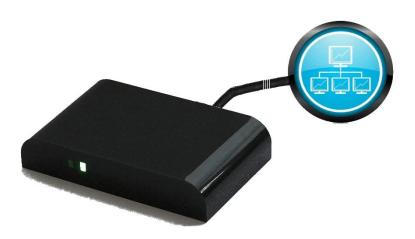
Compatible with the **GESPAGE** server for all network printers, the **Cartadis Tcnet3** reader consists of two cases: the TCM3 USB reader and a CMI-PRINT network interface.
